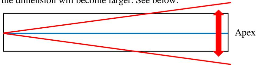
As you can see by the above diagram, the dimension becomes larger as you sweep past the apex point in both directions when on a FLAT standard.
