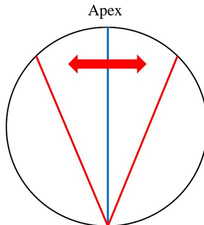
As you can see by the above diagram, the dimensions become smaller as you sweep past the apex point in both directions when on a ROUND surface. While the apex dimension definition alters slightly between measuring on flat and round surfaces, the goal of the gauge is the same. The gauge itself doesn't care whether you are looking for the largest measurement or shortest measurement, it is designed to show you where the apex point is regardless.
